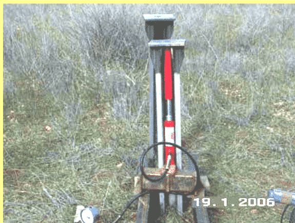
Vertical tension and compression test
